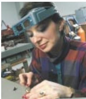
Figure 1 This optivisor provides a magnification up to three times.
