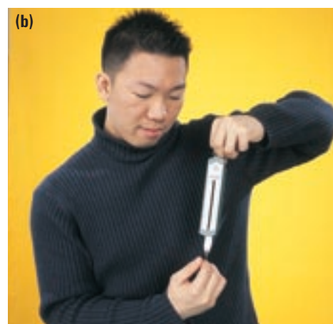
Figure 2 Measuring force in newtons (a) Using a force sensor (b) Using a spring scale
