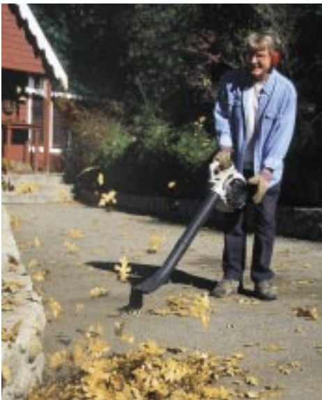
Figure 6 Gasoline-powered blower in operation
