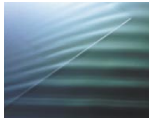
Figure 10 Waves are refracted as they cross a boundary between deep and shallow water if the boundary is at an angle.
