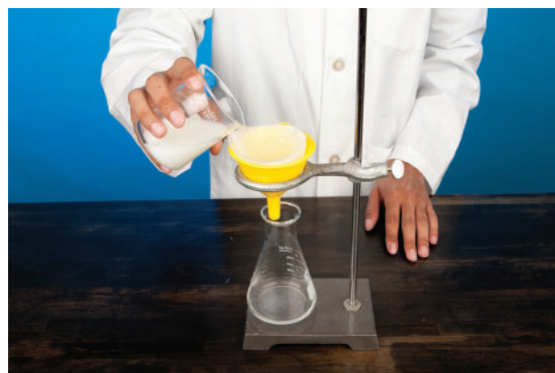
Figure 1 Insoluble substances are trapped in the filter paper.
