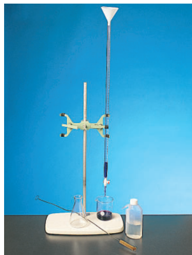
Figure 11 A burette should be rinsed with water and then the titrant before use. Use a burette brush only if necessary.
