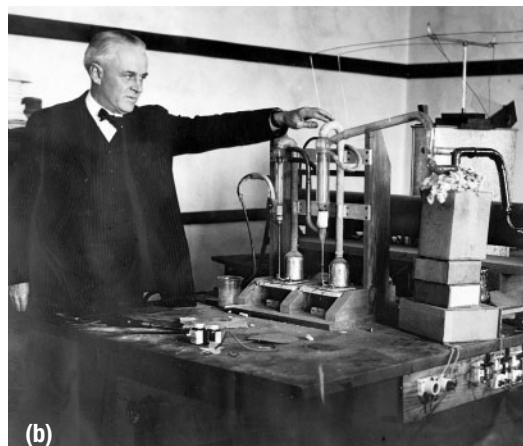
Figure 5 (a) A schematic representation of the apparatus Millikan used to determine the charge of an electron. (b) Robert Millikan using his apparatus
