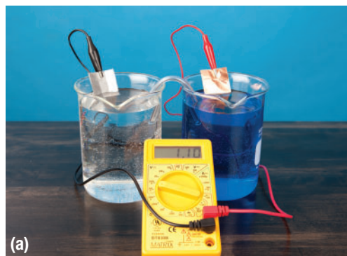
Figure 1 Both (a) an experimental zinc–copper galvanic cell and (b) commercial 1.5 V alkaline dry cells operate on the same principle.
