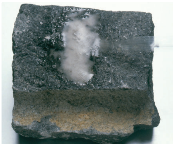
Figure 1 A positive reaction to hydrochloric acid indicates the presence of calcium carbonate in a geological sample.
