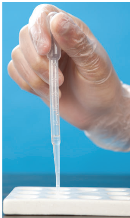
Figure 3 Ensure that the tip of the pipette is below the surface of the liquid.
