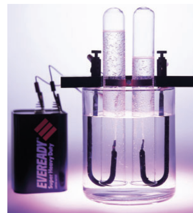
Figure 3 The electrolysis of water produces hydrogen gas at the cathode (on the right) and oxygen at the anode (on the left). Note that twice as much hydrogen as oxygen is produced.
