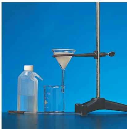
Figure 9 The tip of the funnel should touch the inside wall of the collecting beaker.
