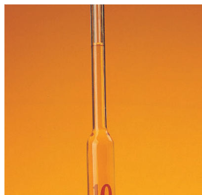
Figure 7 To allow the liquid to drop slowly to the calibration line, it is necessary for your finger and the pipette top to be dry. Also keep the tip on the bottom to slow down the flow.
