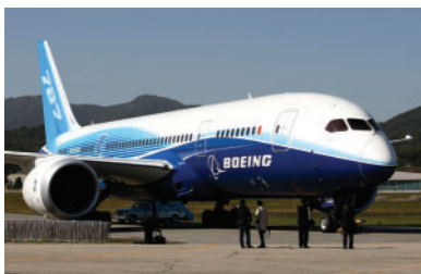
Figure 1 The Boeing 787 Dreamliner, made of composite materials, is more fuel-efficient than older aircraft.
