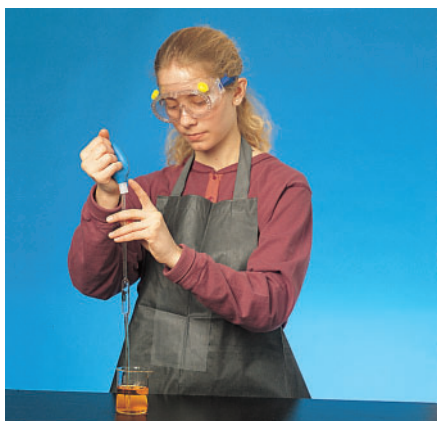
Figure 4 Release the bulb slowly. Pressing down with your thumb placed across the top of the bulb maintains a good seal. Setting the pipette tip on the bottom slows the rise or fall of the liquid.
