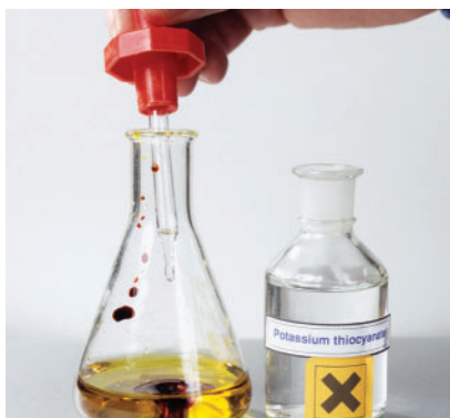
Figure 1 Potassium thiocyanate solution is clear and colourless. When added to a yellow solution of iron(III) nitrate, a deep brownish-red colour is produced, indicating the formation of iron(III) thiocyanate ions. This makes changes in the concentrations of the reactants and products easy to measure with simple equipment.
