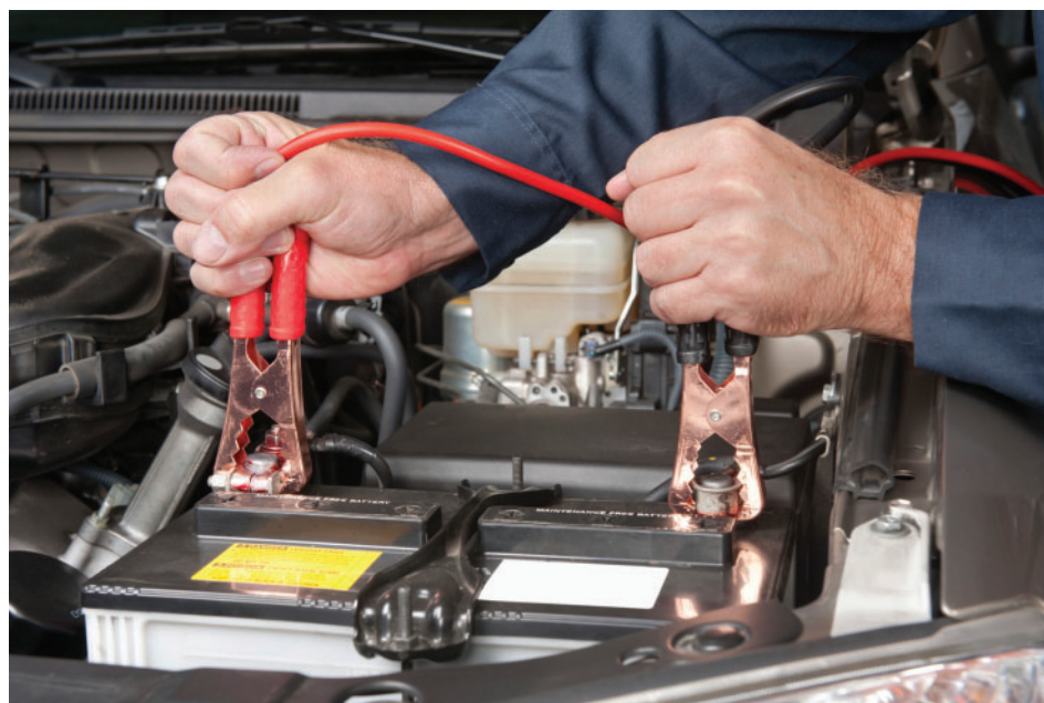
Figure 1 A car with a “dead” battery can be restarted by connecting the dead battery to a working battery. It is important to follow the manufacturer’s directions when setting up jumper cables. Otherwise, a spark might cause the hydrogen gas that is produced to explode.
