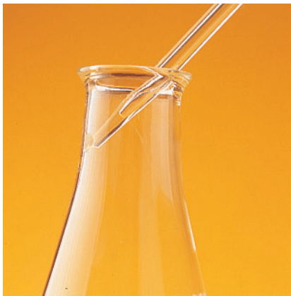
Figure 8 A vertical volumetric pipette is drained by gravity and then the tip is placed against the inside wall of the container. A small volume is expected to remain in the tip.
