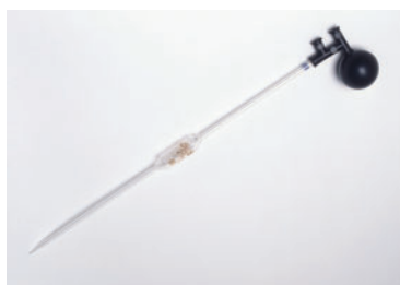
Figure 5 A dispensing bulb uses a small valve in the side stem to control the flow of liquid in a pipette.
