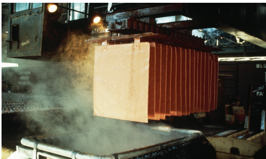
Figure 7 Ultrapure copper sheets, which serve as the cathodes of an electrolytic cell, are lowered between slabs of impure copper, which serve as the anodes. It takes about four weeks for the anodes to dissolve and for the pure copper to be deposited on the cathodes.
