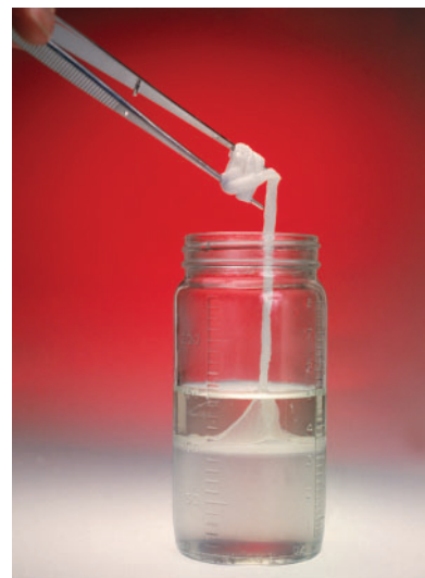
Figure 4 The reaction to form nylon occurs at the interface of two liquid layers in a beaker. The bottom layer is hexanedioyl dichloride dissolved in carbon tetrachloride, CCl 4 . The top layer is hexane-1,6-diamine dissolved in water. A molecule of hydrogen chloride is produced as each C–N bond forms.
