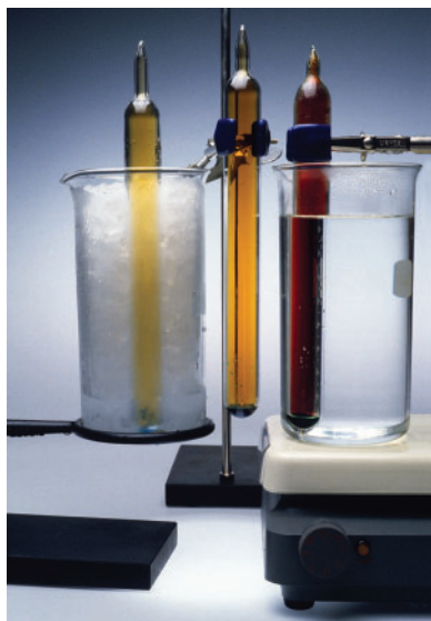
Figure 5 The room-temperature sample in the centre contains a mix of both gases. Changing the temperature shifts the endothermic reaction equilibrium. The sample on the left, at 0 °C, is shifted toward the formation of colourless dinitrogen tetroxide gas. The darker colour of the sample on the right, at 85 °C, is due to a shift toward the formation of reddish brown nitrogen dioxide gas.
