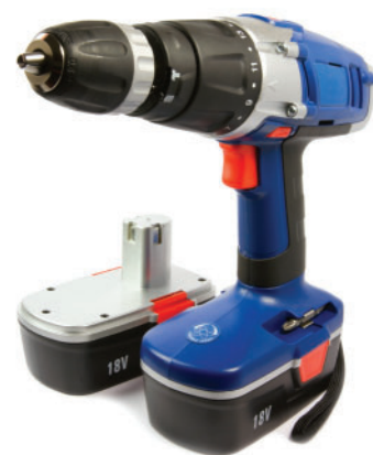
Figure 3 Cordless power tools, such as this drill, use rechargeable batteries. The 18 V battery consists of six 3 V cells connected in series.
