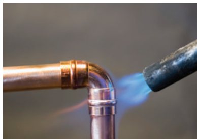
Figure 10 A soldering torch burns propane to produce a flame hot enough to melt some metals.
