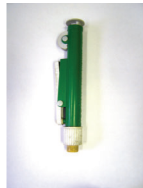
Figure 6 A pipette pump has a small roller that can be turned to draw liquid in or to let liquid out of the pipette.
