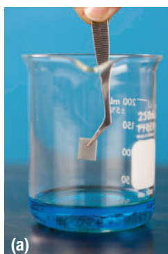
Figure 2 (a) A strip of zinc metal is placed in a solution of copper(II) sulfate. (b) After several hours, the characteristic blue colour of the copper(II) ion, \text{Cu}^{2+}\text{(aq)} , has disappeared, indicating that copper(II) ions are no longer present. Instead, solid copper metal remains in the beaker.
