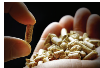
Figure 1 Biomass pellets are primarily cellulose and are made from municipal or agricultural waste. The pellets can be burned directly for fuel or further processed into cellulosic ethanol.
