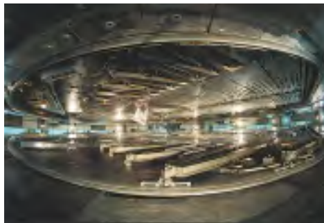
Figure 6 Canada's TRIUMF cyclotron at the University of British Columbia. Charged particles are accelerated around a spiral ring by strong magnetic and electrostatic fields.
