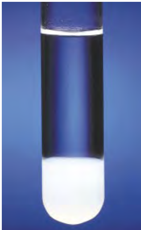
Figure 1 The excess of solid solute in the mixture is visible evidence for a saturated solution.
