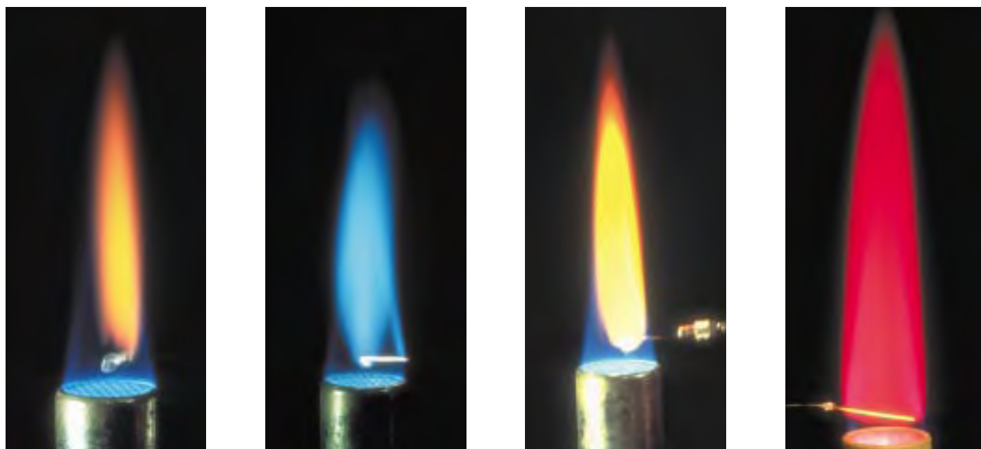
Figure 8 Results of flame tests for four solutions of unknown metallic compounds
