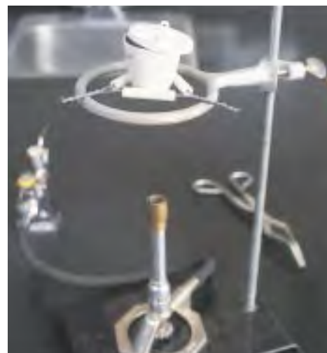
Figure 2 Apparatus for heating in a crucible
