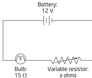
A variable resistor is used to control the brightness of a small light bulb and can be set anywhere from  $0 \Omega$  to  $100 \Omega$ . The total resistance in the circuit is the sum of the resistances of the variable resistor and the bulb.
