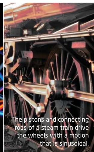
The pistons and connecting rods of a steam train drive the wheels with a motion that is sinusoidal.
