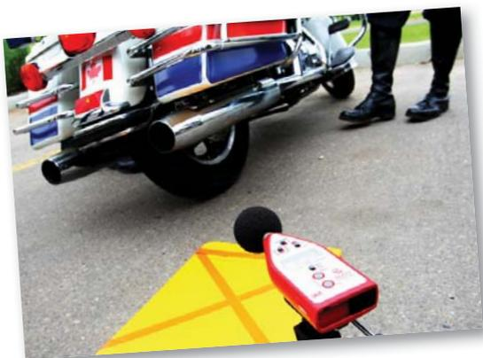
Device used to measure motorcycle noise levels
