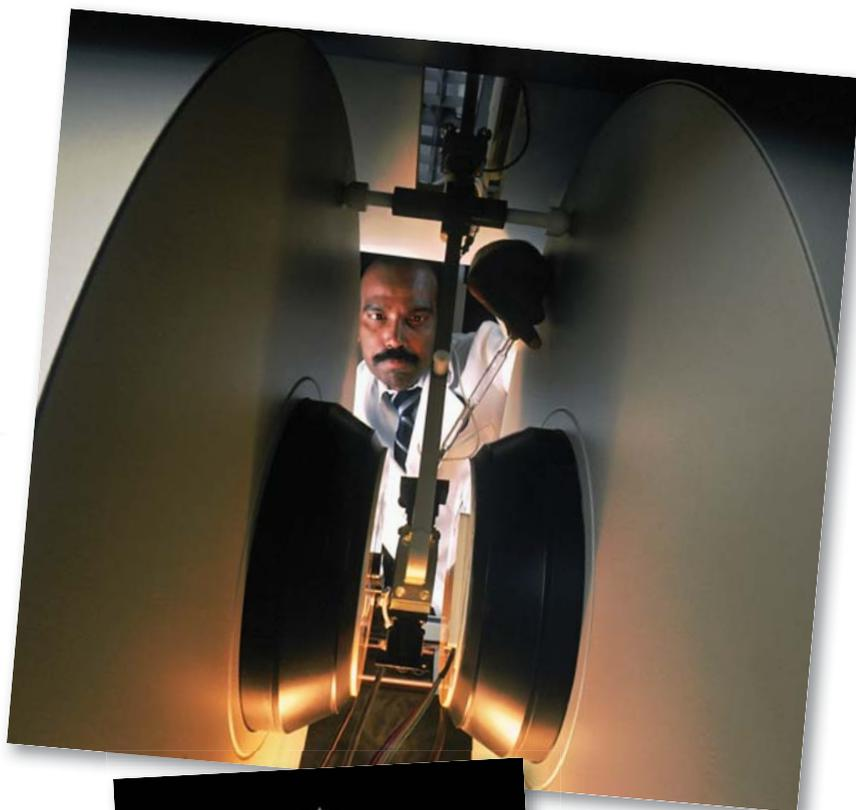
Engineer using an electronic spin resonance spectroscope
